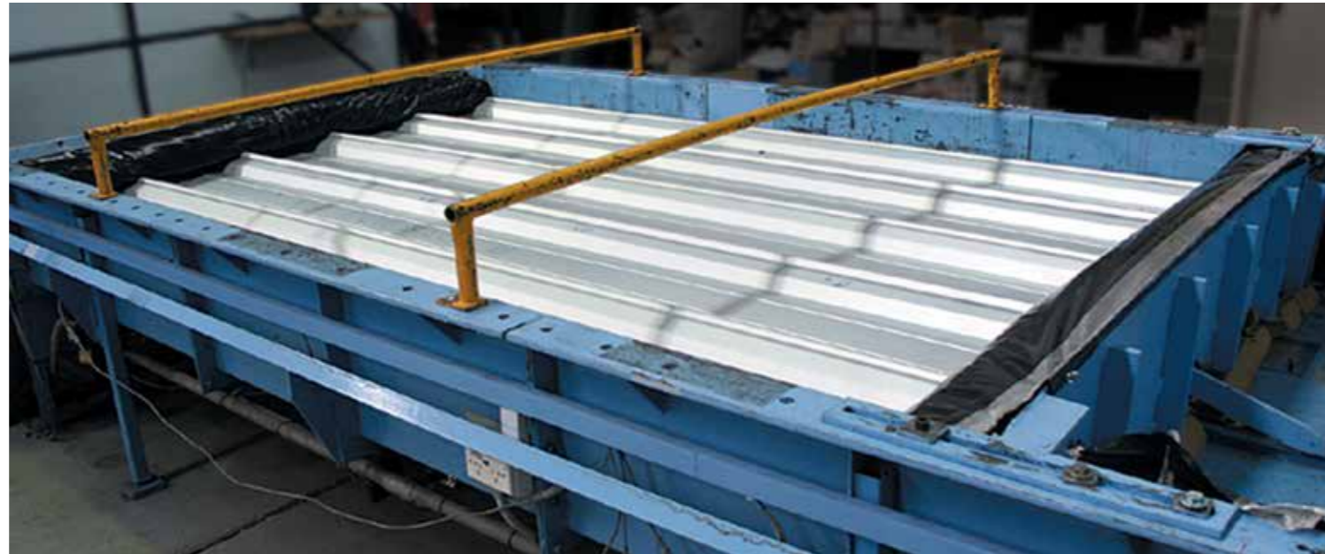
Uniform pressure distribution of our direct pressure rig which accurately reproduces the wind conditions experienced in the field.
