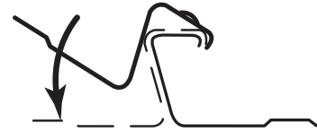
Fig 7.1 Two methods of interlocking adjacent LYSAGHT® BONDEK® II sheets
